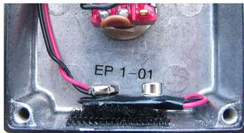
The battery snap is held to the inside of the box with Velcro. Separate the Velcro and attach the snap to the battery. The battery will fit between the switch and the end of the box. The pedal serial number is also located in this area.
