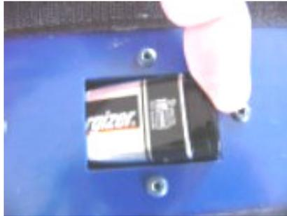
Push battery in against spring and down until the snap clips under the edge
