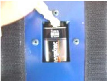
To remove battery, use a small screwdriver, key, coin, thumb nail etc. to push the battery back against the spring, and lift the snap and battery out.
