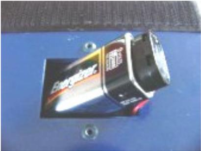
Fit snap to battery and place bottom of battery against spring in battery compartment.
